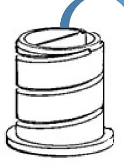
Inner cup with double chamber and screw mechanism (The bottom of the inner container also acts as a lid) Outer container with a screw mechanism that, ensures a comfortable and secure seating of the inner container prevents leakage, and acts as a cup (the base functions as a lid)
